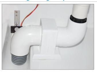
2. Willy Vac: using #14 x 1½" screws, screw down the Willy Vac to the deck.
